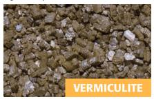
Vermiculite is a micaceous mineral that is expanded in a furnace, forming a lightweight aggregate. It has a good nutrient-holding capacity and provides both air space and water-holding capacity to the mix, along with additional potassium, calcium, and magnesium. Vermiculite tends to be slightly basic. It is a fragile material and can tend to break down with improper or excessive handling. It also can break down over time because of the effect of watering on the media.
